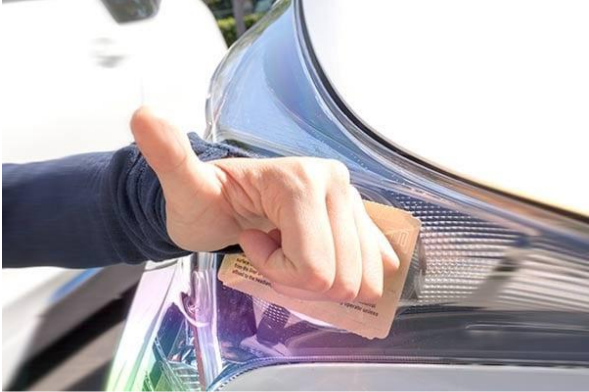
This vehicle has very angular headlights, offering several possible mount points. Pictured above is an upward facing mount point to meet a high mounted antenna.
